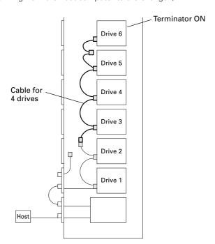
Install 4 internal drives within the changer in a daisy-chain configuration and connect the drives to the changer. (Additional cable for 2 drives will be needed.)
